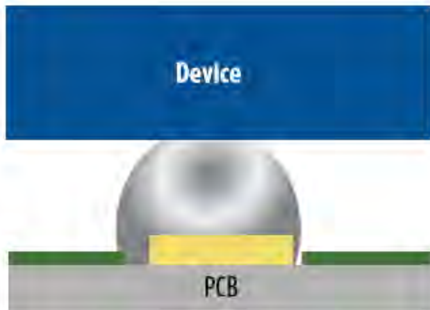
Asymmetrical solder ball (Sensitive to registration) Non-solder mask defined
